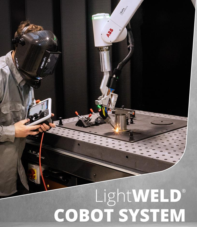
**AUTOMATED** LASER WELDING & CLEANING
