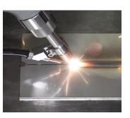
Used for laser wire welding of low carbon steel, stainless steel, aluminum, non-ferrous metals & other alloys. Wire feeder nozzle attachment guides wire precisely to the weld pool. Light**WELD** Process Modes provide standard parameter settings for typical materials and wire types.
